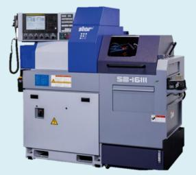
CNC Swiss Type Automatic Lathe SB-16III
