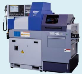
CNC Swiss Type Automatic Lathe SB-16III
