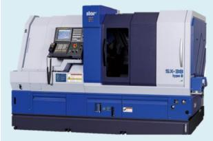
CNC Swiss Type Automatic Lathe SX-38 type B
