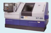
CNC Swiss Type Automatic Lathe ST-20
